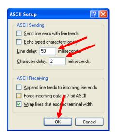
Set the *Line delay* to 50 millisecond. This is the delay between each command.
