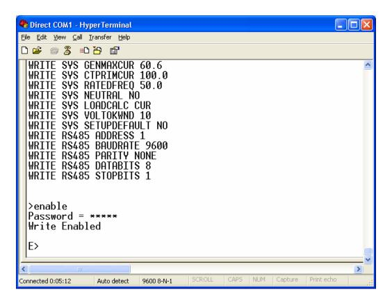
Once the password is entered, the module will acknowledge the entry into READ/WRITE mode with an "E" in front of the prompt. The module can be switched back to READ ONLY mode using the disable command.
