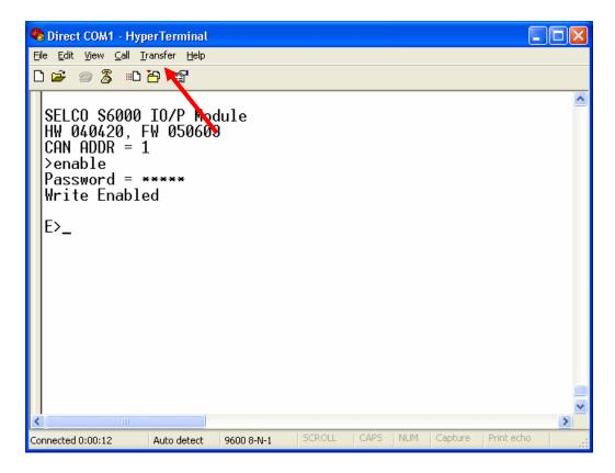
Enable the module for READ/WRITE access using the ENABLE command (default password is 0000). Then Left click on the *Transfer* menu.
