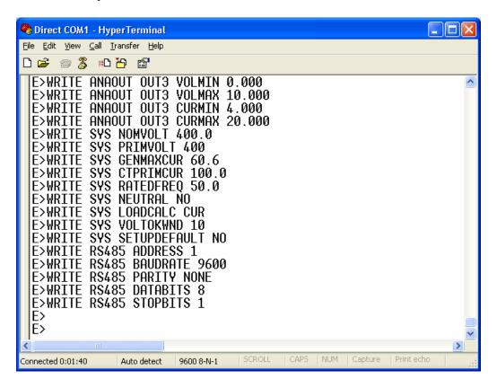
This causes the content of the text file (S6000 Config.txt) to be written back into the Sigma module – line by line.
