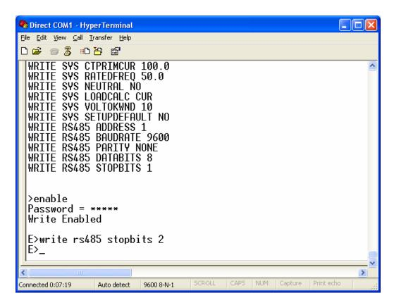
Now type the command WRITE RS485 STOPBITS 2 at the prompt and hit the ENTER key.
