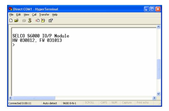
The HyperTerminal application will start and the Sigma module (in this case an S6000 IO/P module) will acknowledge the connection with a short welcome message and a ">" prompt. The prompt indicates that the module is ready to receive a command.
